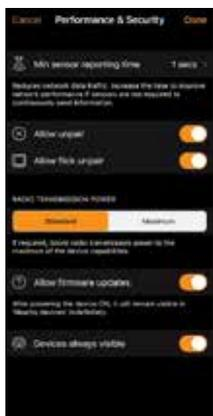
**Min sensor reporting time** defines how often lux sensors report values to the network. Choosing a higher interval reduces network traffic, especially in networks with many sensors.
