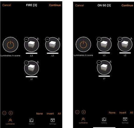
... a small icon (triangle with an exclamation mark inside) in the top right of each luminaire will indicate the Emergency priority command is affecting the luminaire.
