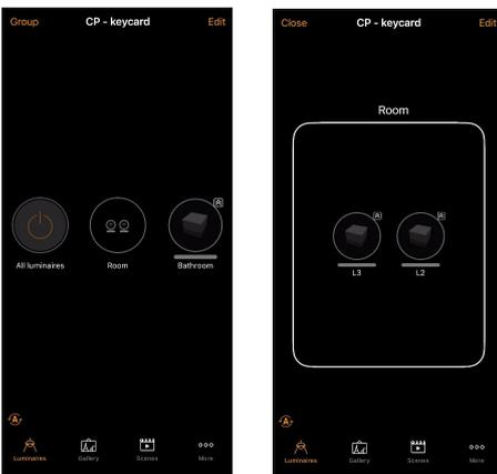
... a small icon (square with two upward-pointing arrows inside) in the top right of each luminaire will indicate the **Higher than manual** command is affecting the luminaire.
