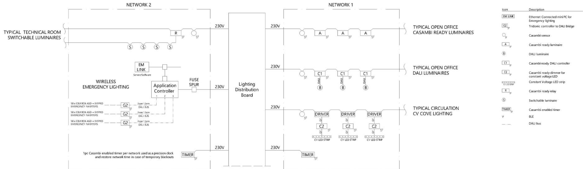
NOTE: Casambi Evolution networks contain up to 250 nodes (luminaires, sensors, switches) depending on the selected network mode. Casambi Evolution networks with DALI Emergency integration can contain up to 64 Casambi nodes. There is no limit to the number of networks.
